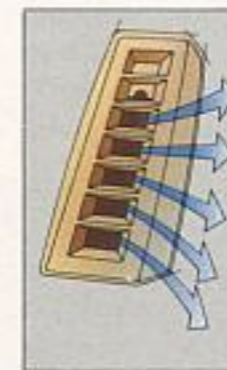
The newly incorporated side window demisters help keep the side windows free of condensation.
