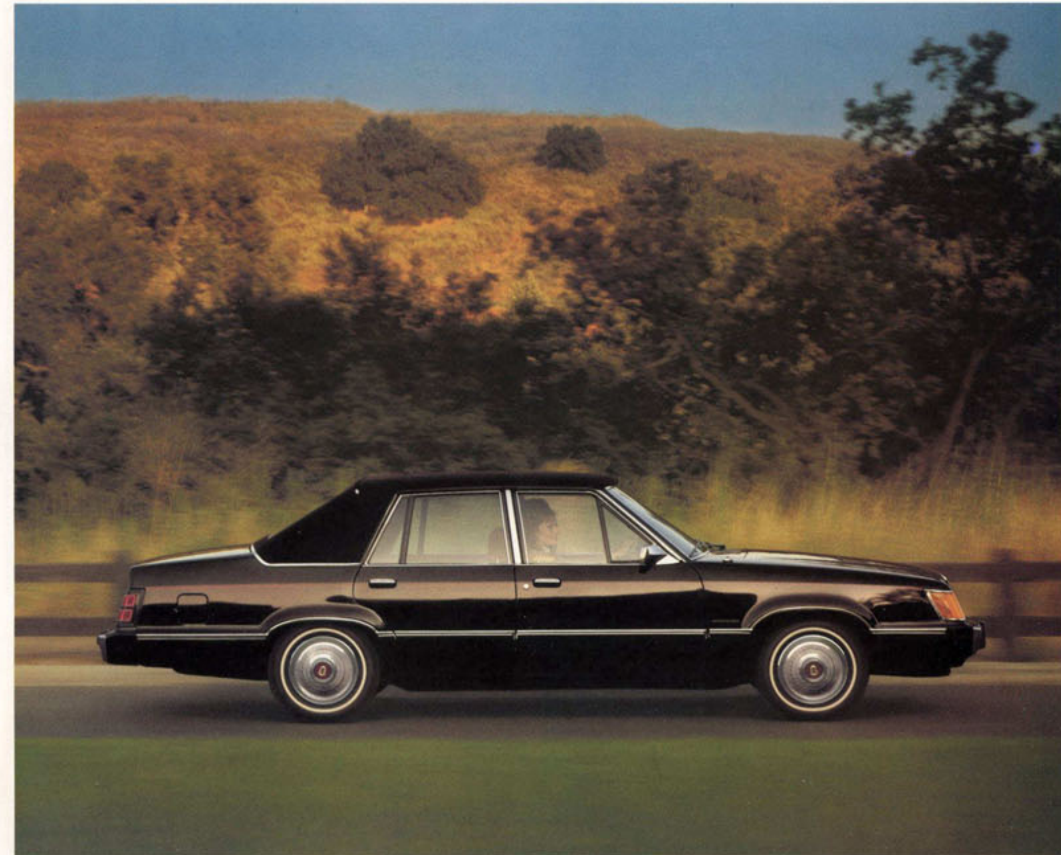
LTD Brougham 4-Door Sedan shown with optional right-hand convex remote-control mirror, pivoting front vent windows, wire-style wheel covers and white sidewall tires.
