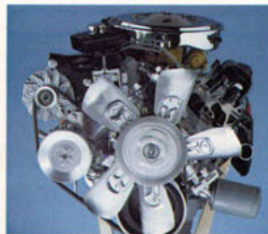
3.8 liter V-6 engine (chrome added for display purposes only).
