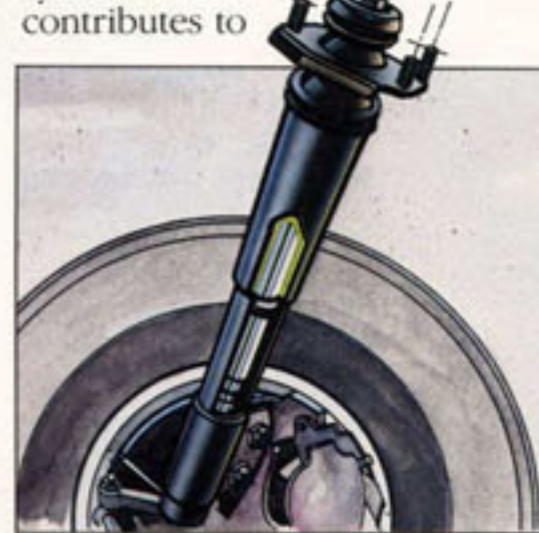
Gas-filled shock absorbers are designed to handle the full range of road surfaces and driving situations.
