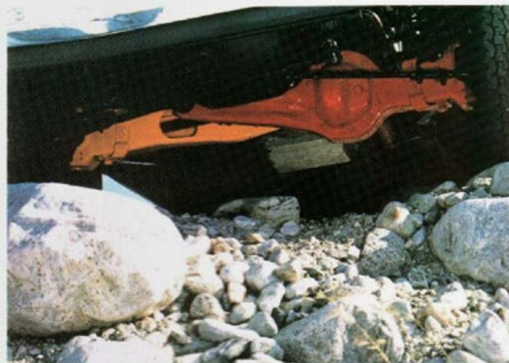
Above: Twin-Traction Beam independent front suspension. (Some items are painted for display purposes.)
