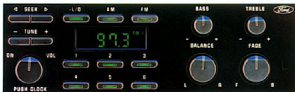
Electronic AM/FM stereo search radio, standard with Thunderbird and Thunderbird Super Coupe.
