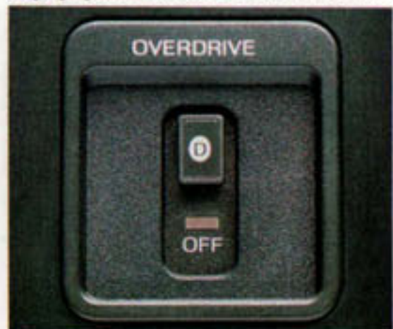
▲ E4OD Overdrive Cancel Switch inhibits upshift to overdrive gear at the driver's discretion — a real plus in heavy-duty applications like trailer towing.
