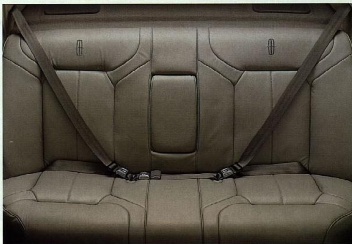
Outboard rear passengers are provided with lap/shoulder safety belts. The center rear passenger is provided with a lap belt.
