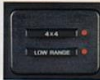
The push-button controls for the standard Touch Drive electric shift transfer case are on the instrument panel — a more convenient arrangement than the floor-mounted shift found in other 4x4 pickups. A manual shift transfer case with manual locking front hubs is available in place of Touch Drive.
