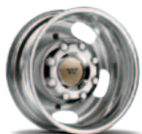
17" Polished Forged-Aluminum Standard: F-350 DRW/F-450
