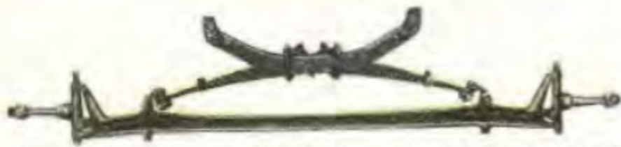
Front axles on all Model T Cars are each drop-forged from one single ingot of Vanadium steel specially heat-treated in our own plant
