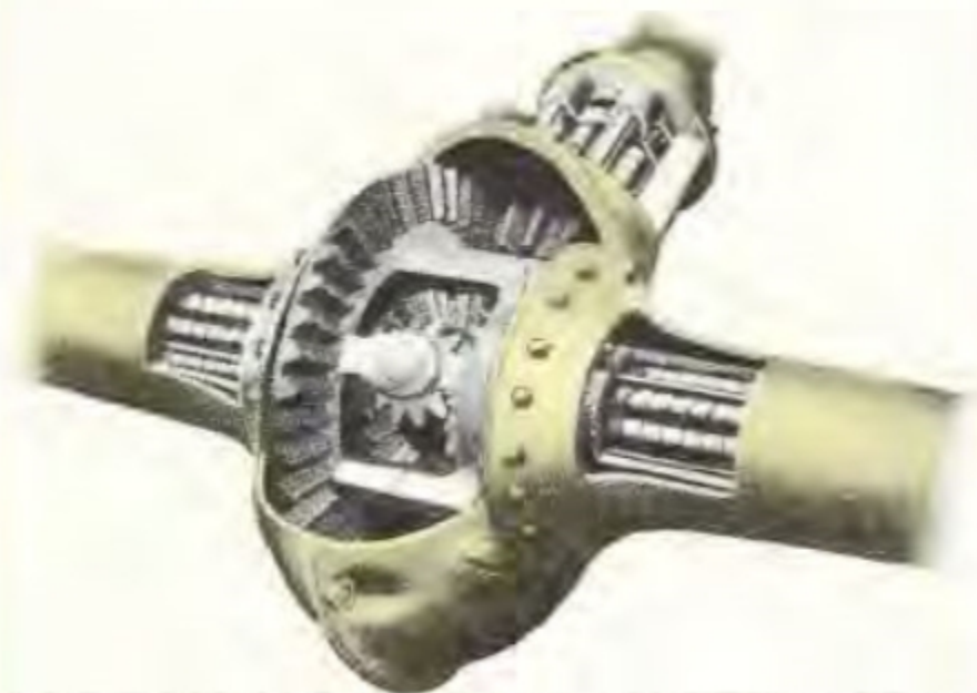
Three pinion bevel type Model T differential, noted the world over for its simplicity and smooth running
