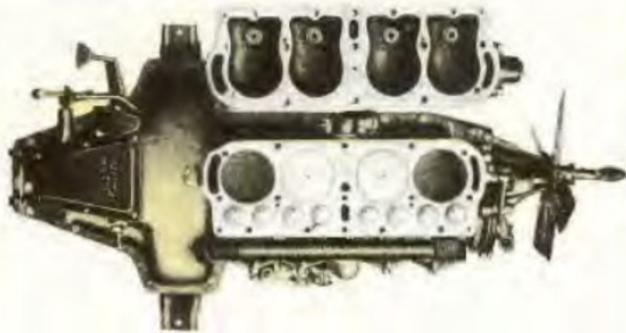
Top View of Motor, with cylinder head removed, showing pistons, valve setting, and water jackets
