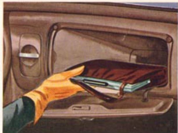
A large compartment, located on either side of the instrument panel, provides a convenient place for gloves, sun glasses, small packages and maps. One is equipped with a lock.
