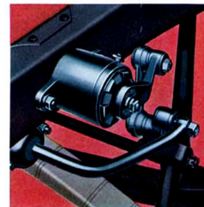
LIKE A GIANT'S HELPFUL HAND , a newly perfected stabilizer helps hold the body level, adds to riding comfort.
