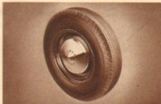
New Low Pressure Tires . . . 6.70 x 15 . . . available at extra cost on all models except station wagon, for an even smoother ride! (7.10 x 15 6-ply low pressure tires are standard on station wagon.)
