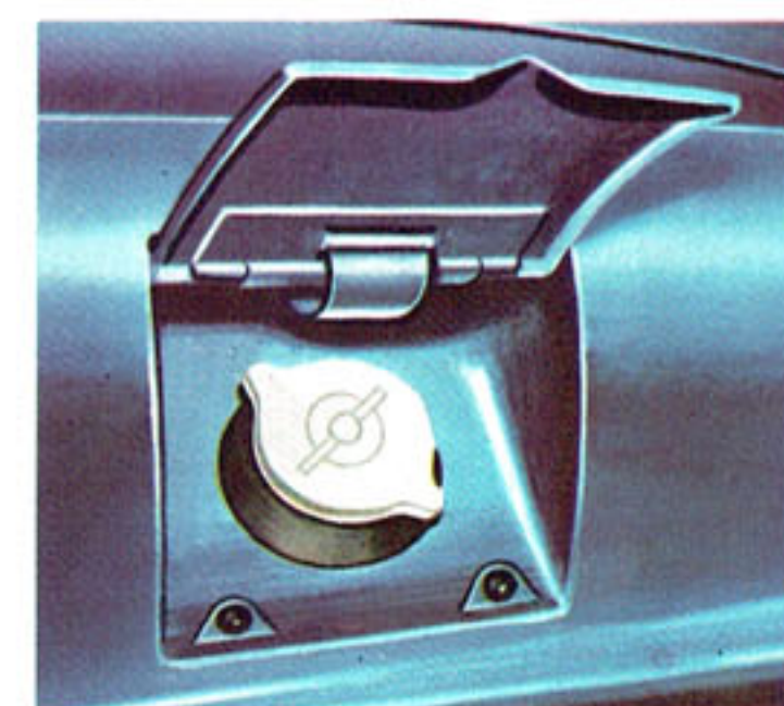
New Gas Filler Tube and Cover. New vent tube helps prevent spilling. Cover is flush with body when closed.
