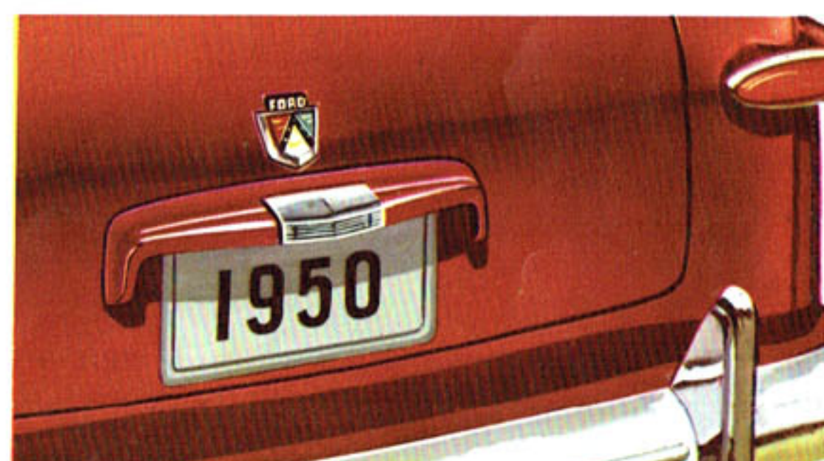
New Deck-Lid Handle incorporates new trigger-type latch. Makes attractive frame for license plate. Permits easy access to roomy, weather-sealed luggage compartment.
