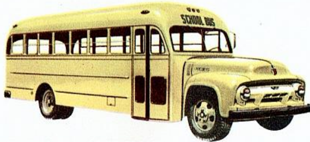
B-600 SCHOOL BUS CHASSIS WITH BODY 192-in. wb., up to 54-passenger loads. 210-in. wb., 55-passenger loads.
