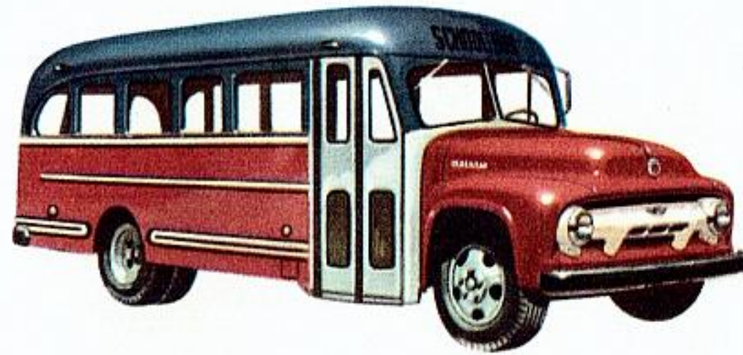
B-500 SCHOOL BUS CHASSIS WITH BODY 154-in. wb., up to 36-passenger loads.
