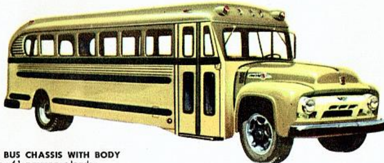
B-600 SCHOOL BUS CHASSIS WITH BODY 192-in. wb., up to 54-passenger loads. 210-in. wb., 55-passenger loads.
