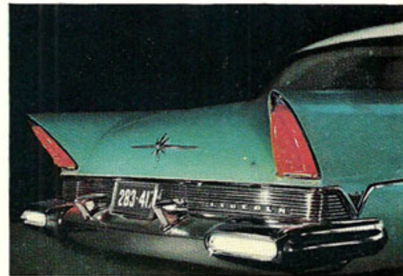
Powerful back-up lights are housed in the wrap-around bumper, cast more light over a broader area than do those of any other car. They illuminate to the side, as well as to the rear.
