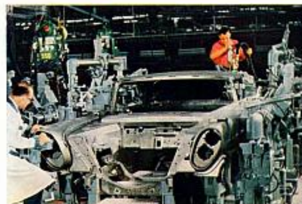
Here in our new plant, you see quality craftsmanship at its finest. In this single gigantic framing jig, for example, entire Continental and Lincoln bodies are checked and welded to closer tolerances. The building and inspection of a body and frame unit is a completely integrated operation that results in a new kind of solid silence and strength.
