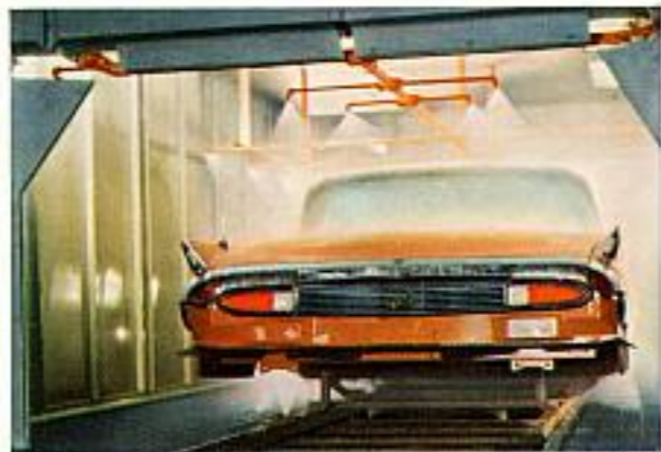
Every Continental and Lincoln body receives a severe water test. In this spray booth, 36 nozzles—each exerting 24 pounds of water pressure—shoot water at windows, doors, trunk lid and virtually —every point where water could seep in. An inspector inside the body checks for any possible leaks, and they are corrected immediately.
