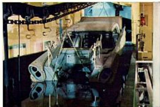
Here's the kind of beneath-the-surface quality you won't find in any other fine car. We use an entirely new rust-inhibiting system ... an improvement over the conventional spray-on method. Bodies are immersed to the belt line in a huge pool filled with a special paint—where hidden parts receive protection against rust and corrosion.
