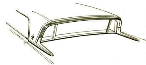
Retractable rear window—the kind of advanced feature you expect in Continental. Just flick a switch on the driver's armrest control panel and the rear window slides out of sight—to give you open-car ventilation. (On all Continental models, including the Convertible.)
