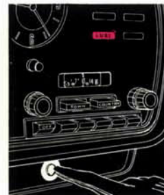
Touch —and you have Power Lubrication as you drive. In just a matter of seconds, a green light indicates the front suspension and steering system have been completely lubricated.
