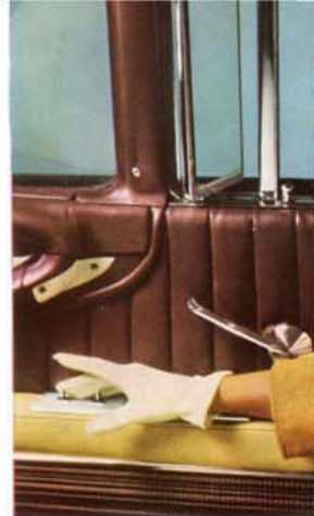
Touch . . . and power vent windows let you adjust ventilation without taking your eyes from the road. A switch on the driver's door controls both vents, and a switch on the opposite door lets passengers operate the right-hand vent.
