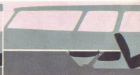
2 2nd seat folds forward and flush with floor (same as in 4-door models—explained below) when you need additional loading area.
