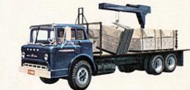
Tilt Cab Tandem Axle Series . . . now you can get the servicing and handling ease of Ford's modern tilt-cab design plus tandem-axle haulability in four factory-engineered Tilt Cab Tandems. These extra-heavy-duty models are available on a special order basis in GVW's from 35,000 lb. to 51,000 lb. with GCW ratings up to 75,000 lb.
