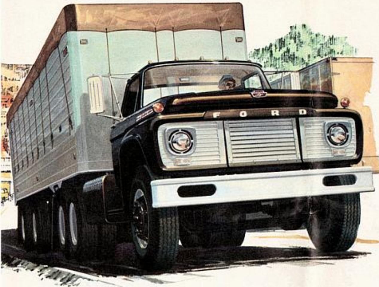
T-850 tractor with axle-forward design provides a short 102-inch BBC to haul longer high-cube trailers. High-tensile steel frame provides strength for durability and lightweight design for maximum payloads.
