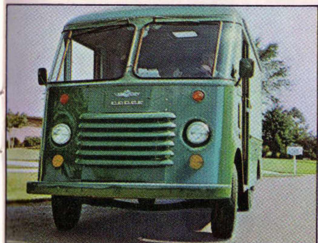
DODGE P300. Available on 104", 125" and 137" wheelbase lengths, with GVW ratings to 10,000 lbs. Powered by a Dodge 225-1 Slant Six engine.
