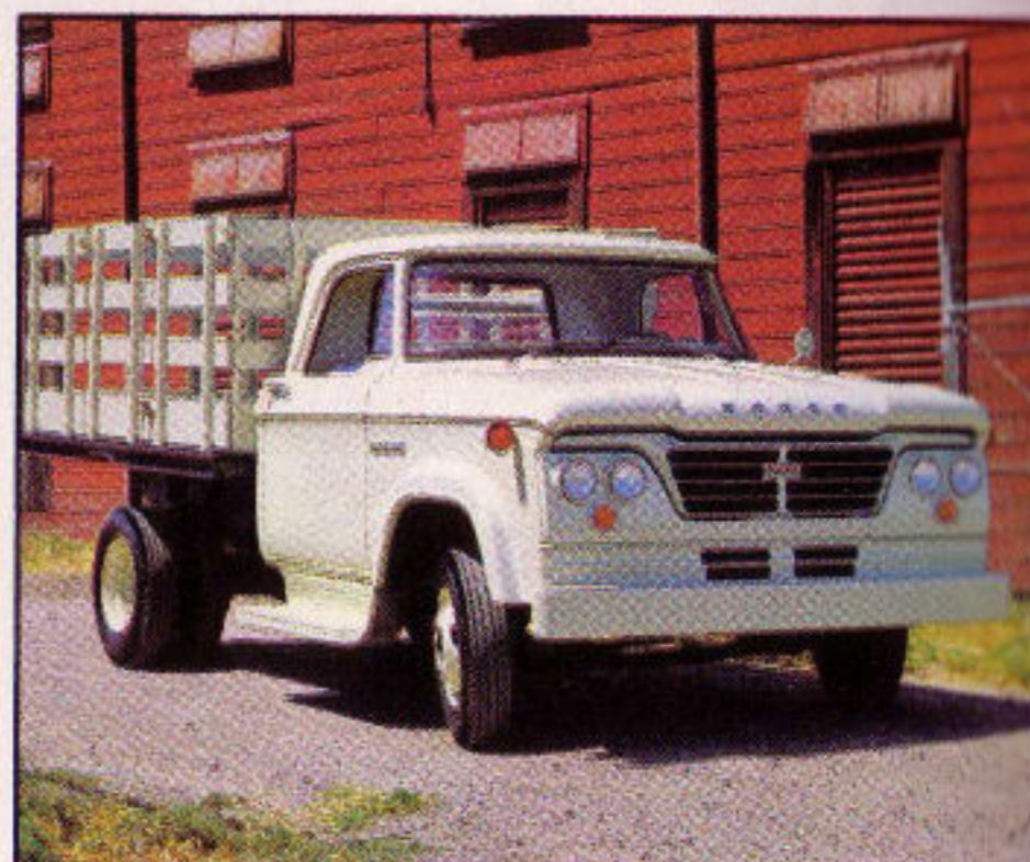
DODGE STAKES. Three models on two wheelbase lengths. GVW ratings go to 10,000 lbs. Hardwood flooring with steel sills.
