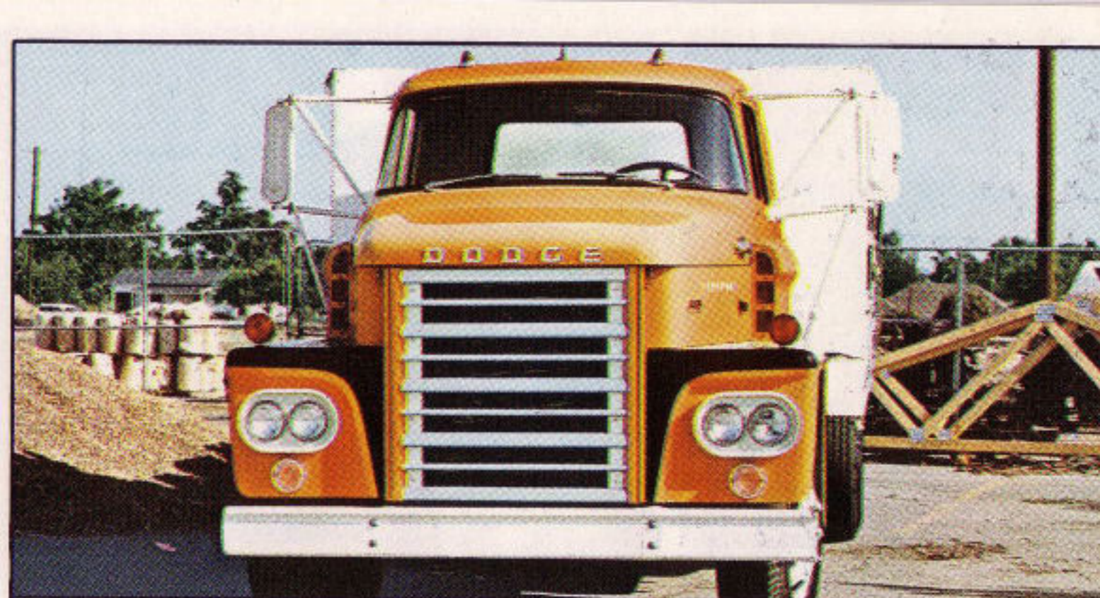
DODGE DIESEL PC600. Another 89 \frac{3}{4} " BBC, with a GVW rating of 22,000 lbs., and a GCW rating of 36,000 lbs. Engine is a 354 cu. in. Dodge-Perkins diesel. Transmission is a 4-speed New Process 433.
