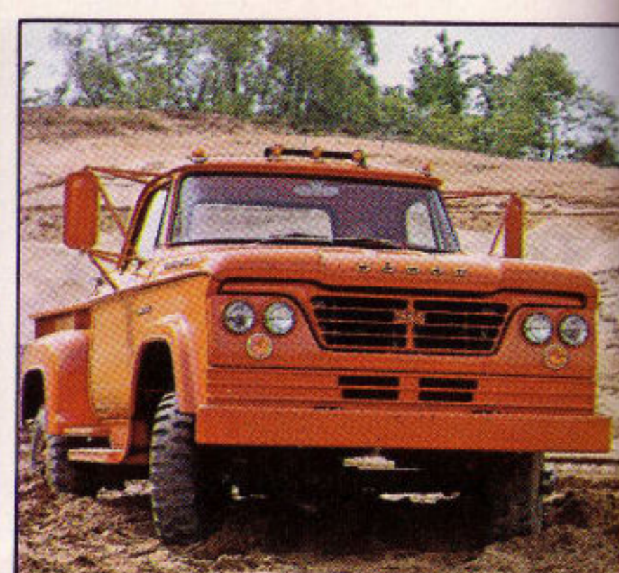
DODGE W300 UTILINE. With 9-foot box on a 133" wheelbase. Comes with either 8,500 or 10,000 lbs. GVW rating.
