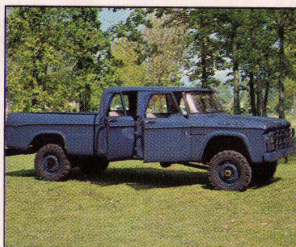
NEW DODGE CREW CAB. Available with 6½-foot Sweptline or Utiline pickup body on 146-inch wheelbase W200 chassis.
