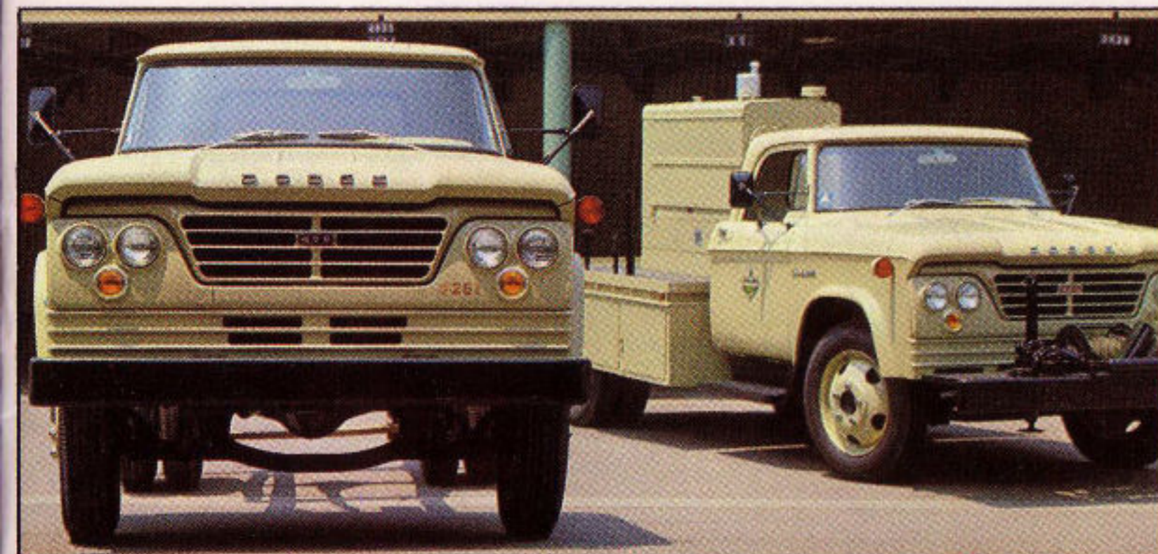
DODGE D400. A thrifty worker in the 15,000 lb. GVW, 25,000 lb. GCW range. Powered by the 140 hp Dodge 225-2 premium Slant Six engine, with a 318 cu. in. V8 optional for maximum performance.
