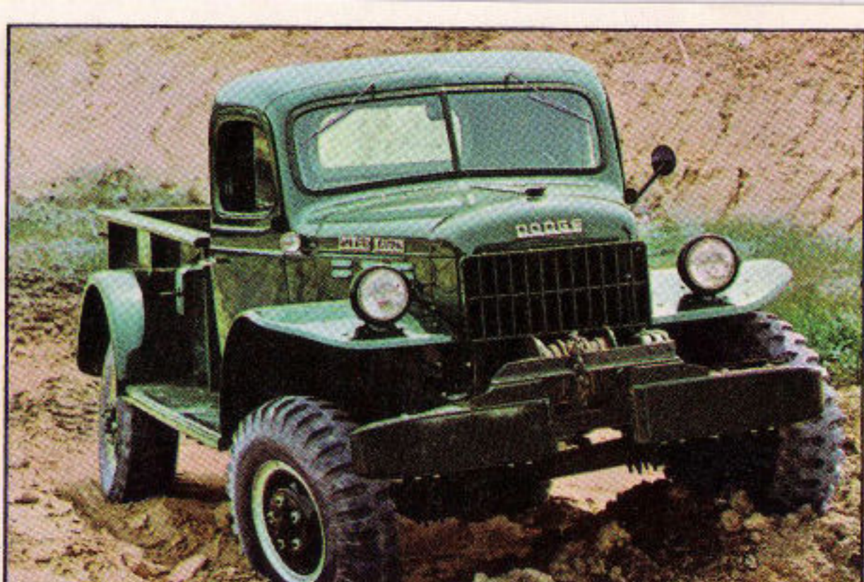
DODGE WM300 MILITARY TYPE. A famous model with an 8-foot Utiline body on a 126" wheelbase. Also available as chassis-cab.
