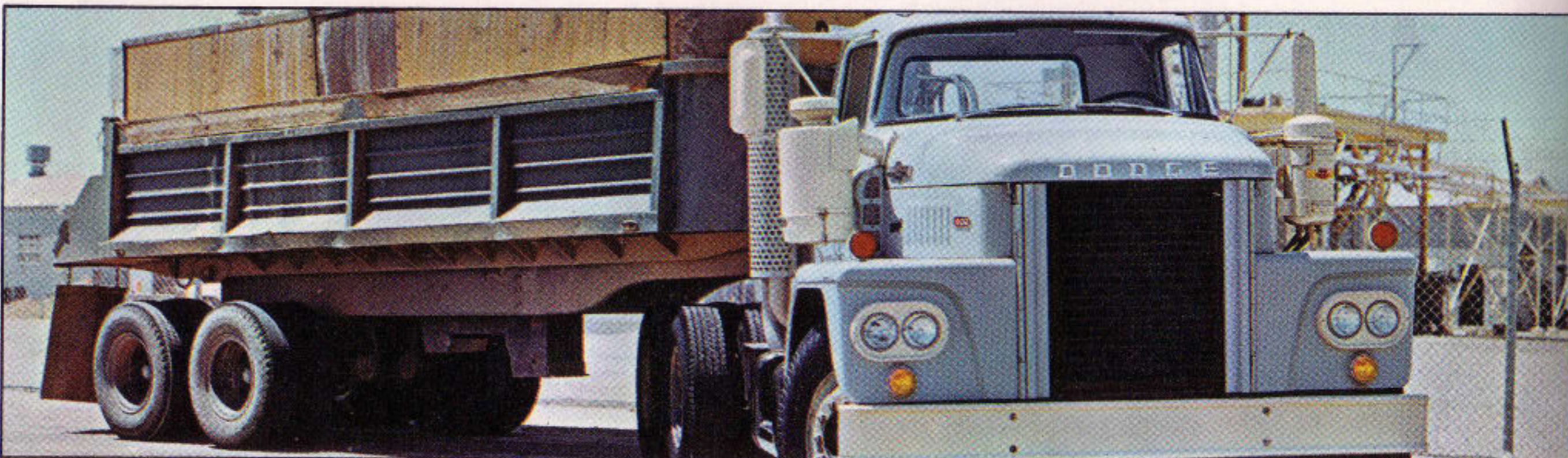
DODGE DIESEL NCT900. Rated at 49,000 lbs. GVW, 70,000 lbs. GCW. Powered by a Cummins NH-180 diesel engine, with a 5-speed Spicer model 6452A transmission.
