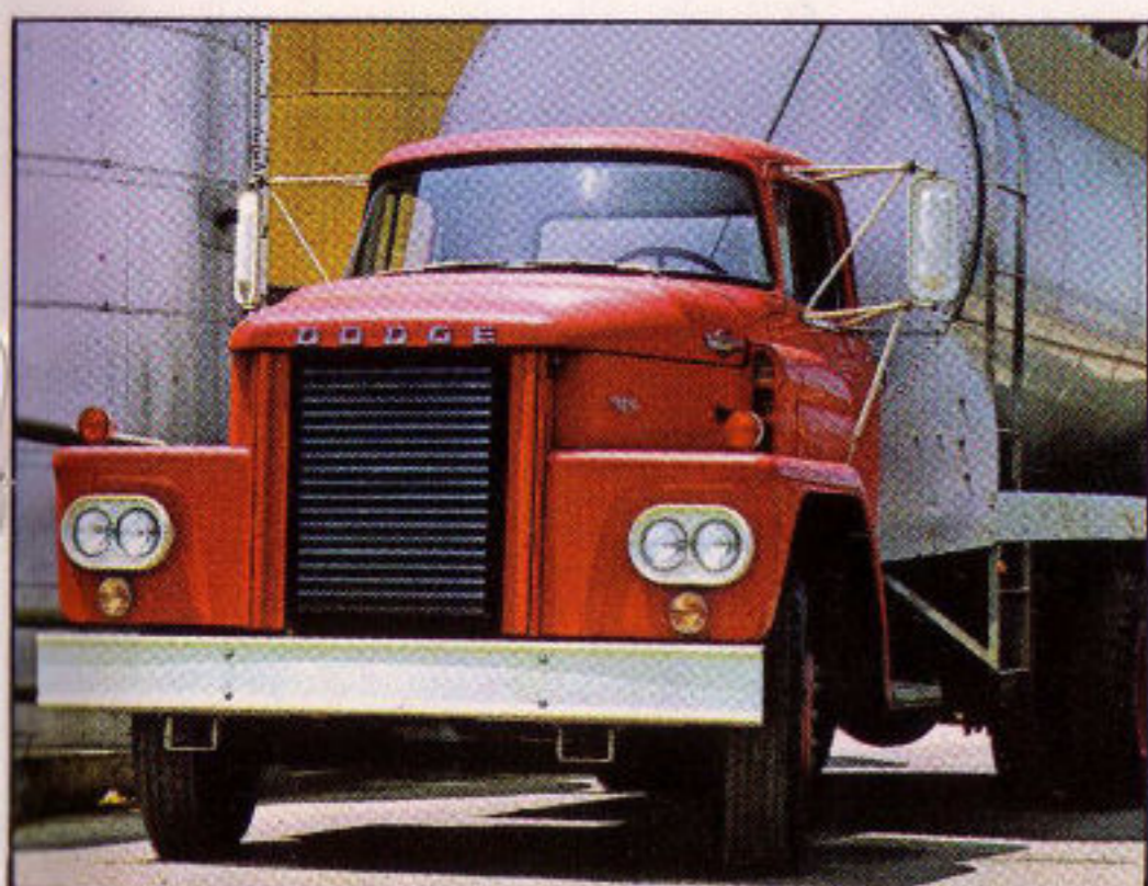
DODGE CT700. A tandem model with a GVW rating of 39,000 lbs., GCW rating of 55,000 lbs. Engine is a 361 cu. in. V8.
