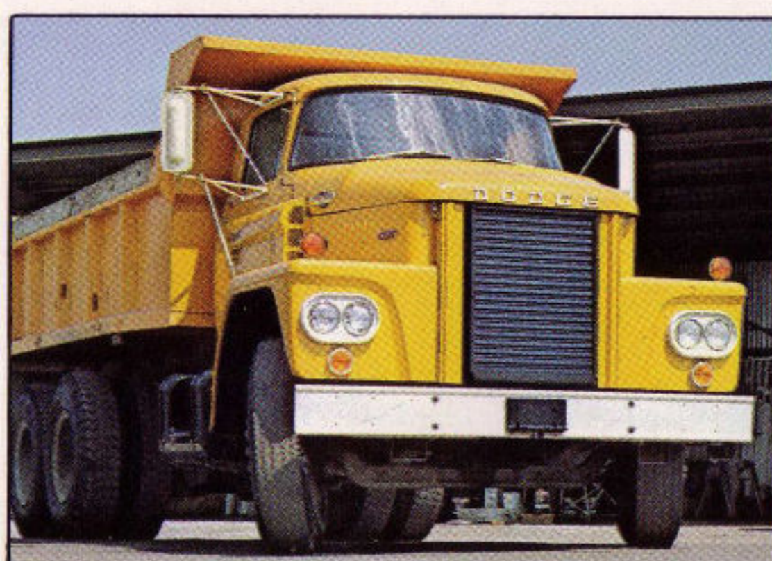
DODGE CT800. A tandem model with a GVW rating of 45,000 lbs., a GCW rating of 60,000 lbs. A 361 cu. in. V8 is standard.
