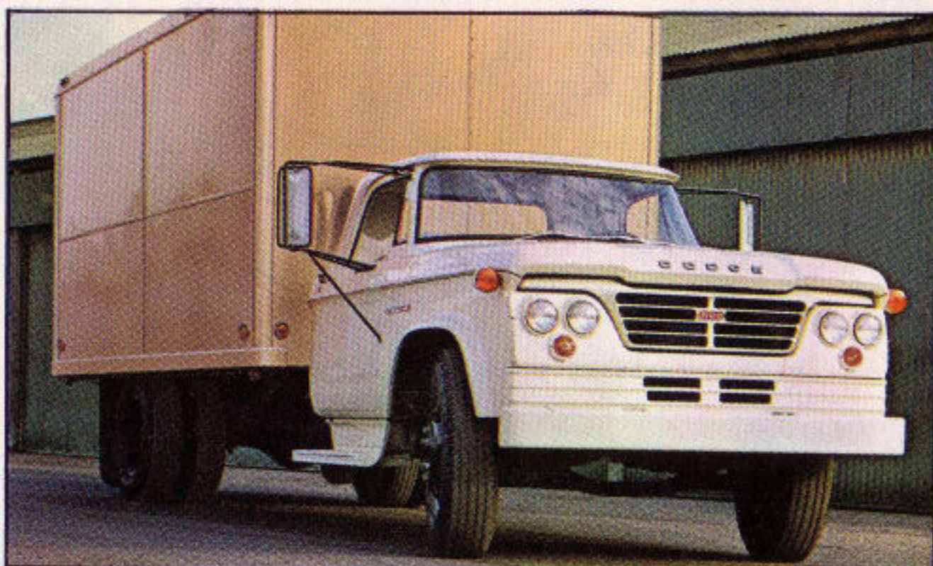
DODGE DIESEL PD500. A conventional cab model with a GVW of 19,500 lbs., a GCW of 34,000 lbs. Powered by a 354 cu. in. Dodge-Perkins diesel engine, with NP 433 4-speed transmission.
