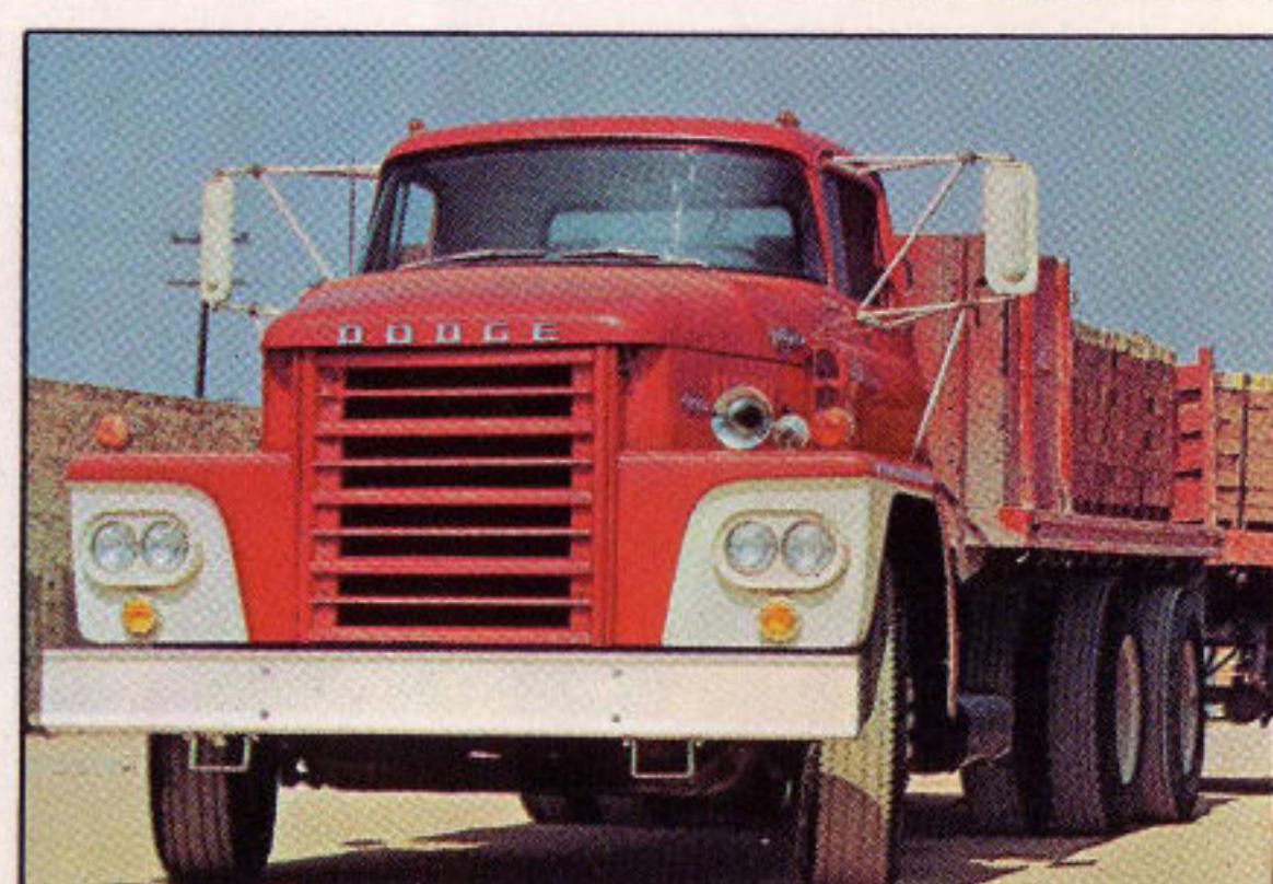
DODGE CT900. A tandem model rated at 53,000 lbs. GVW, 65,000 lbs. GVW, 65,000 lbs. GCW. Powered by a rugged, heavy-duty 413 cu. in. V8.
