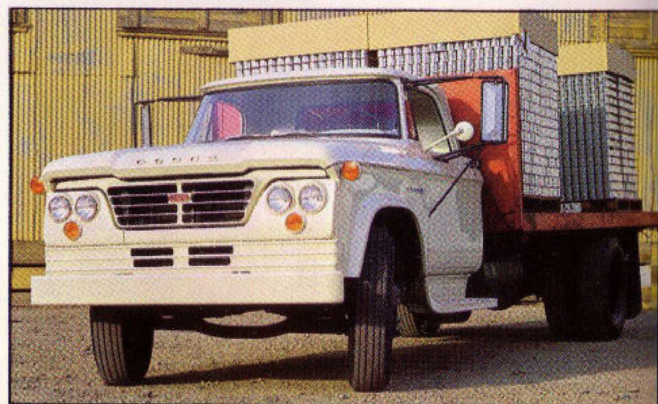
DODGE D500. With a GVW of 19,500 lbs., and a GCW of 34,000 lbs. Powered by the 140 hp Dodge 225-2 Slant Six; 318 cu. in. or 361 cu. in. V8 engines optional.
