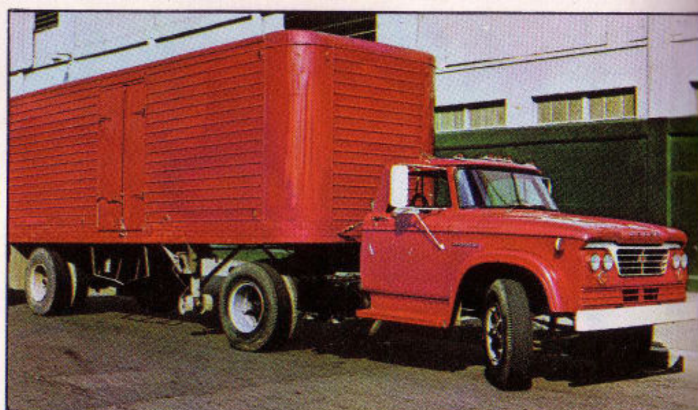
DODGE DIESEL PD600. Rated at 22,000 lbs. GVW and 36,000 lbs. GCW. Engine is a 354 cu. in. Dodge-Perkins diesel. Standard transmission is a 4-speed New Process Synchro-Shift model 433.
