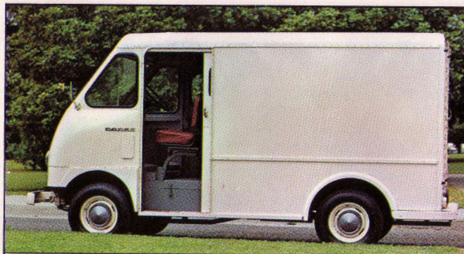
DODGE P100. With a maximum GVW of 5100 lbs. on a 104" wheelbase. Standard engine is a 225-1 Slant Six. Options include a 170 cu. in. Six for use where economy is more important than performance.
