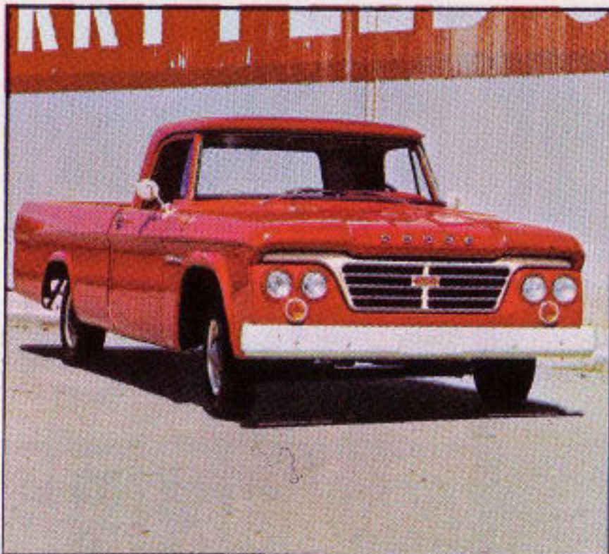
DODGE SWEPTLINE PICKUPS. With a 6½-foot box on 114" wheelbase, 8-foot box on 122" wheelbase. Six or V8 engine.
