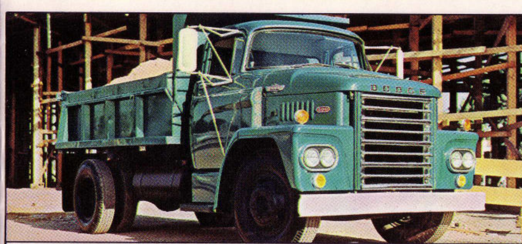
DODGE DIESEL PC500. With a BBC of 89 \frac{3}{4} " , a GVW rating of 19,500 lbs., and a GCW rating of 34,000 lbs. Powered by the 354 cu. in. Dodge-Perkins diesel engine, with a New Process 433 4-speed transmission.
