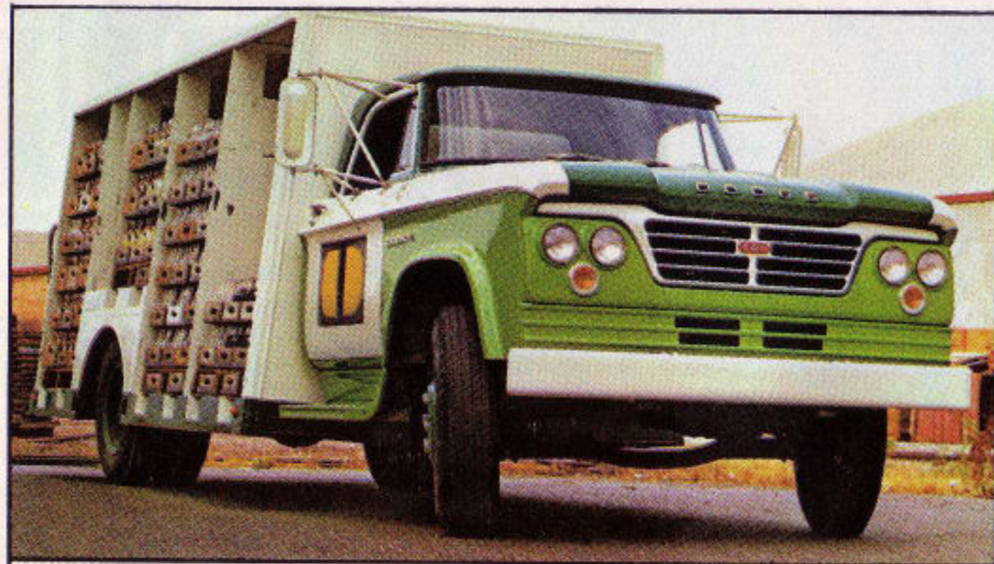
DODGE D600. Rated at 22,000 lbs. GVW, 36,000 lbs. GCW. Powered by a 318 cu. in. V8 engine, with a premium heavy-duty 361 cu. in. V8 engine optional. Full air brakes are optional equipment.
