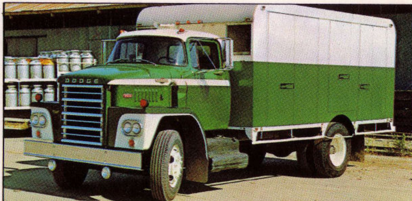
DODGE C700. Rated at 25,000 lbs. GVW, 50,000 lbs. GCW. Powered by a heavy-duty 361 cu. in. V8 engine, with a 5-speed transmission and 17,000 lbs. rear axle standard equipment.
