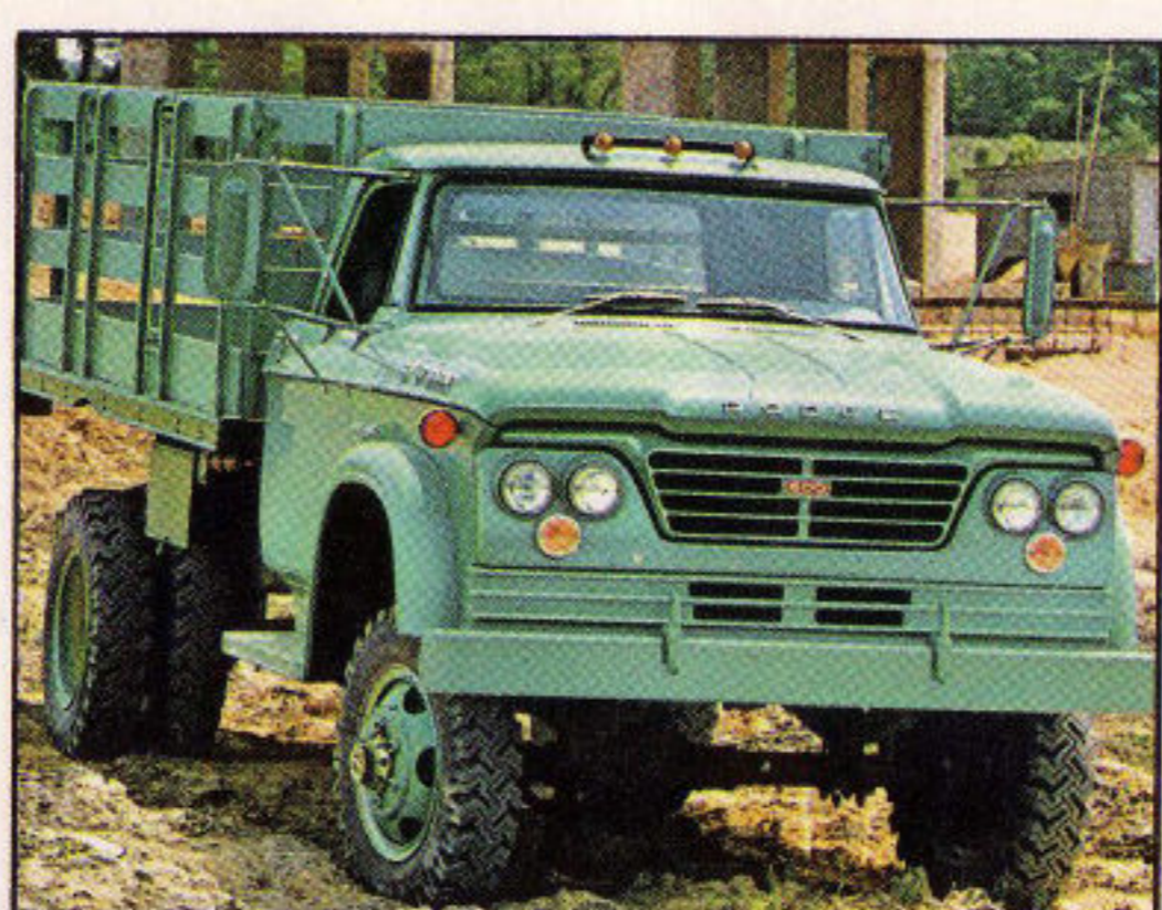
DODGE W500 STAKE. Model W500, with 84" and 102" cab-to-axle dimensions, can be fitted with a wide variety of bodies.
