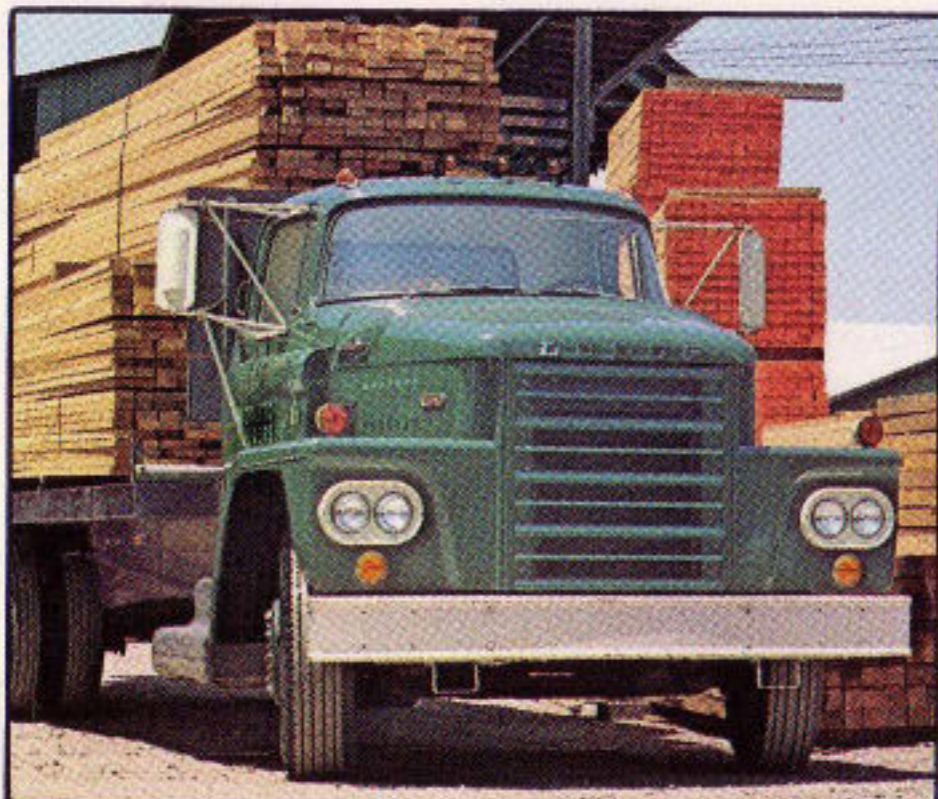
DODGE C800. With a GVW rating of 28,000 lbs., GCW rating of 55,000 lbs. Powered by a tough, economical 361 cu. in. V8 engine.
