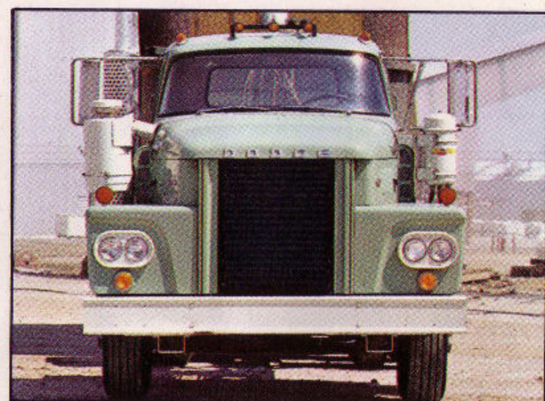
DODGE DIESEL NCT1000. 53,000 lbs. GVW, 76,800 lbs. GCW. Powered by a Cummins NH-220 diesel engine. Also tandem diesel model NCT800.
