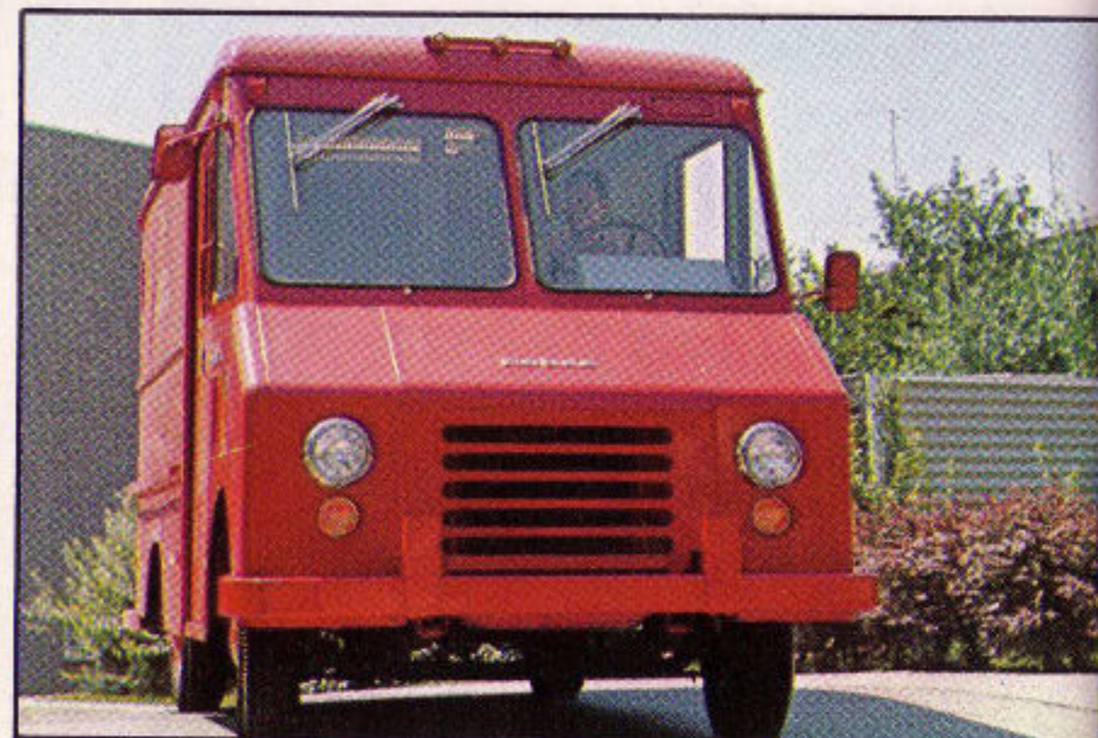
DODGE P200. On two wheelbase lengths—104" and 122"—with GVW ratings to 7500 lbs. Standard engine is a 225-1 Slant Six. Options include a 170 cu. in. Slant Six.
