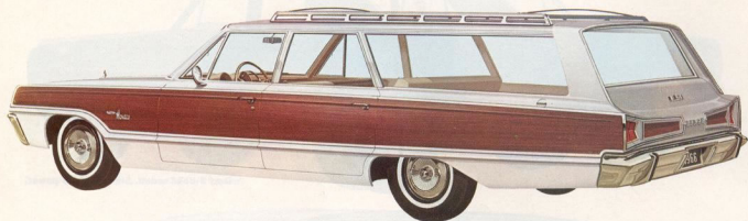
Monaco station wagon. Finest wagon Dodge builds. 121-inch wheelbase, simulated walnut paneling, 383 V8 power are standard. 2- and 3- seat models.
