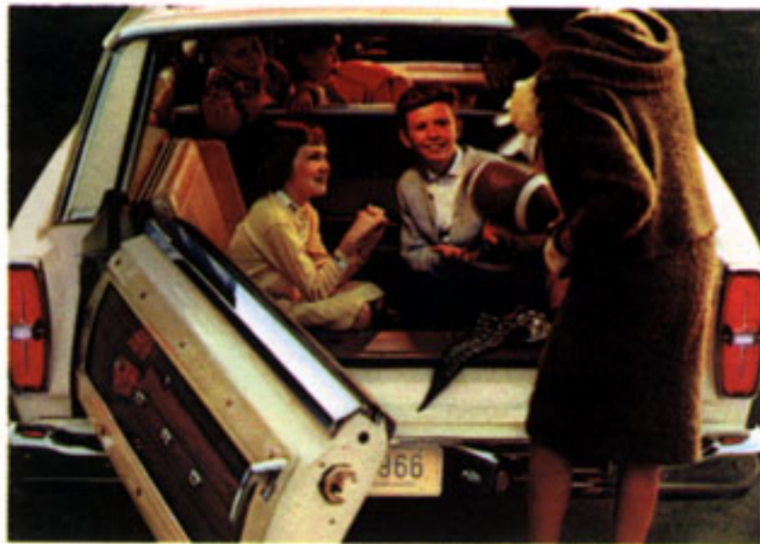
Now it's a door . . . for easier entry or close-up loading. New Magic Door is shown on the '66 Ford Country Squire. Notice the dual-facing rear seats in this model.
