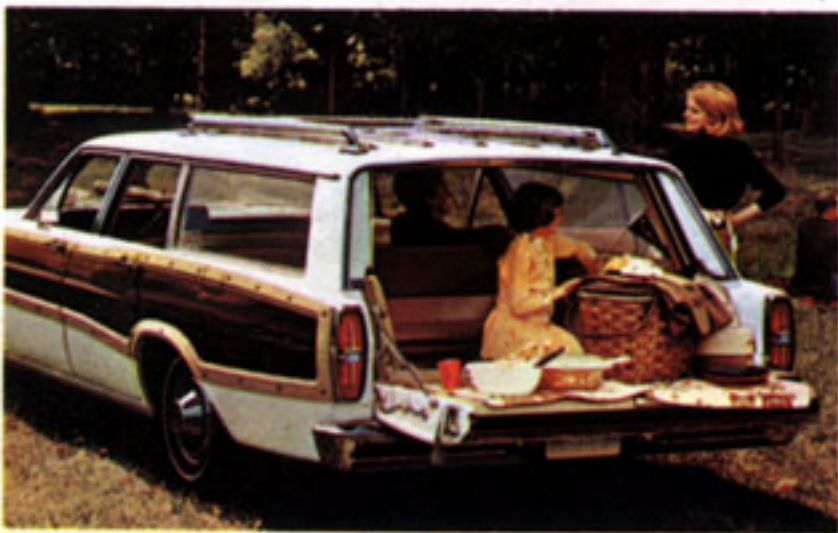
Now it's a tailgate! Used as a conventional tailgate, the Magic Doorgate extends the loadspace for long cargo, can also serve as a platform or picnic table.
