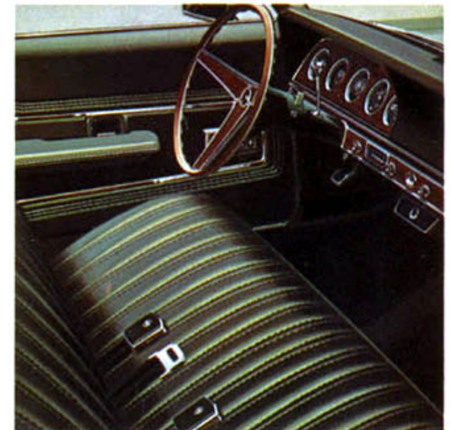
All-vinyl standard Cyclone interior with optional Rim-blow steering wheel
