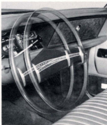
Standard steering wheel for Imperial; optional on all other Chrysler models. Features rim-blow steering wheel and 2 spokes with padded center.
