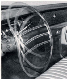
Standard steering wheel for all Chrysler models except Imperial. Features wood-grained insert at center, 3 spokes and horn tabs on spokes.
