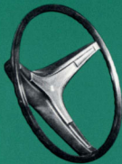
Standard steering wheel for all Chrysler models except Imperial. Features wood-grained insert at center, 3 spokes and horn tabs on spokes.
