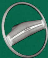
Optional Tilt-A-Scope Steering Wheel has straight-through spoke with padded center and rim-blow horn.
