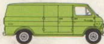
E-300 SuperVan 123.5-in. wb., 8300-lb. max. GVW clear floor length: 123.7 in.
