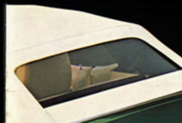
CONVERTIBLE POWER-OPERATED TOP is of padded, 5-ply vinyl. Solid, tempered-for-strength glass backlite resists scratching, won't fade or discolor.
