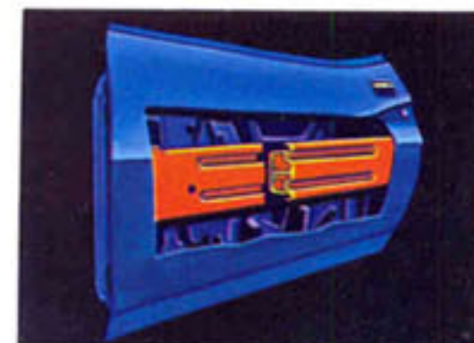
Sturdy steel guard rails are built into doors.
