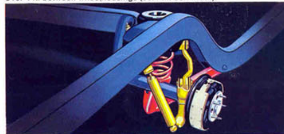
New link-coil rear suspension (coil springs with angle-mounted upper and lower stabilizer arms) smooths and stabilizes for better handling, remarkable roadability.
