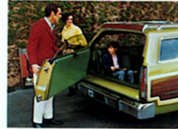
3-WAY MAGIC DOORGATE. Opens as a door... window up or down, and folds down as a tailgate. It simplifies cargo and passenger loading and is standard—along with power tailgate window—on all Ford wagons.
