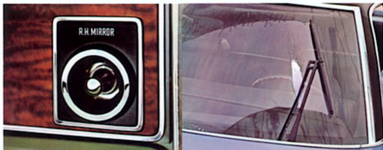
CONVENIENCE GROUP. Includes six handy items: remote control left hand and right hand mirrors—adjustable from driver's seat for best rearview without opening window; automatic parking brake release (see illustration on facing page); interval windshield wipers—let you regulate pause between sweeps from 2 to 10 seconds to handle road splatter, light rainfall, for best visibility. Visor vanity mirror—recessed into reverse side of right-hand sun visor; and auxiliary ash tray in right front armrest. Also illustrated: new standard wiper-mounted washer jets to direct fluid precisely where needed.
