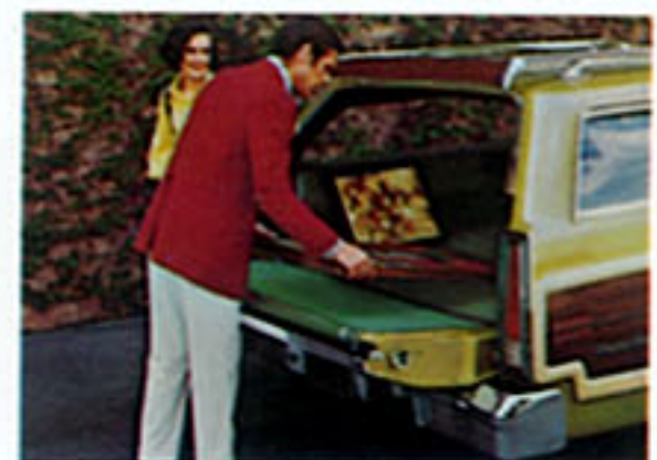
3-WAY MAGIC DOORGATE. Opens as a door... window up or down, and folds down as a tailgate. It simplifies cargo and passenger loading and is standard—along with power tailgate window—on all Ford wagons.
