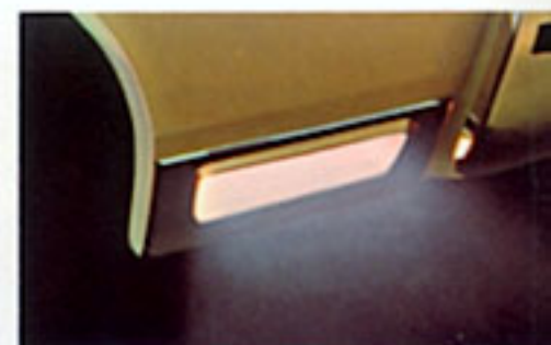
FRONT CORNERING LAMPS (LTD Broughams, LTD's, Country Squires) light up dark turns, work with turn signals.
