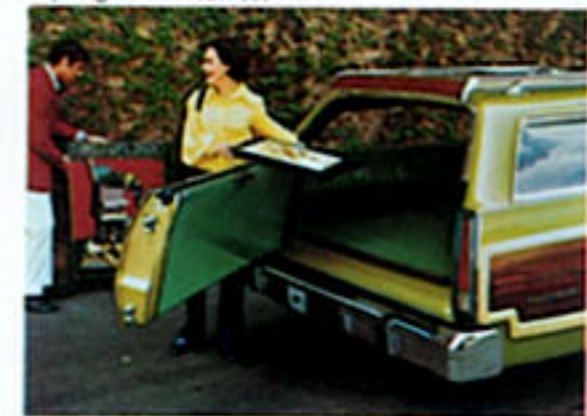
3-WAY MAGIC DOORGATE. Opens as a door... window up or down, and folds down as a tailgate. It simplifies cargo and passenger loading and is standard—along with power tailgate window—on all Ford wagons.
