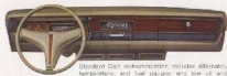
Standard Dart instrumentation includes alternator, temperature, and fuel gauges, and low oil and brake-on warning lights.
