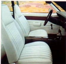
Optional Dart Sport interior includes a floor-mounted automatic transmission, cassette, and all- vinyl bucket seats in black or white.
