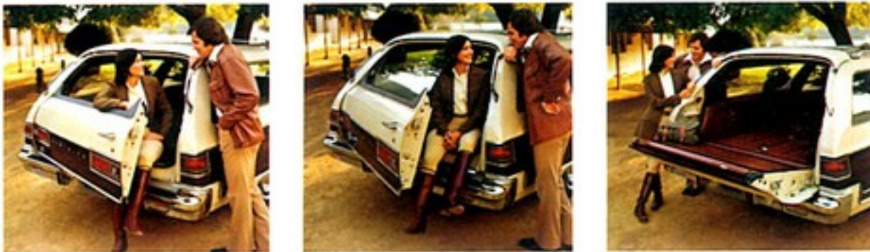
Three-way doorgate is standard. When dropped down, doorgate is almost level with cargo floor for easy loading.
