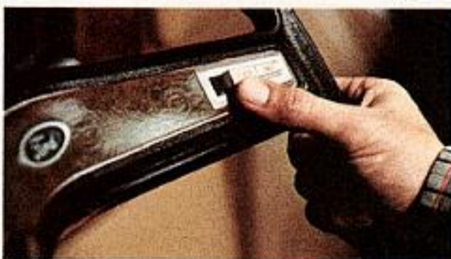
SelectShift Cruise-O-Matic transmission allows fully automatic or manual shifting.
