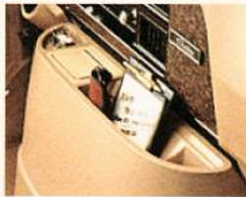
Molded, insulated engine cover console.
