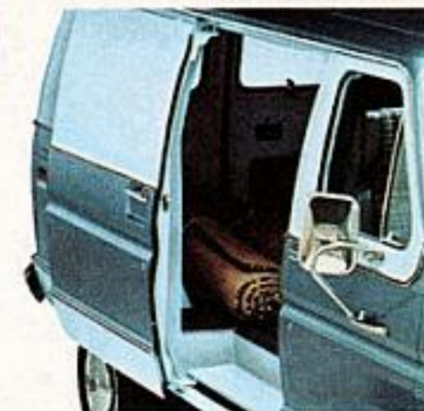
Sliding side cargo door allows easy cargo handling in narrow alleys and against loading docks. Convenient, weather-protected inside step.
