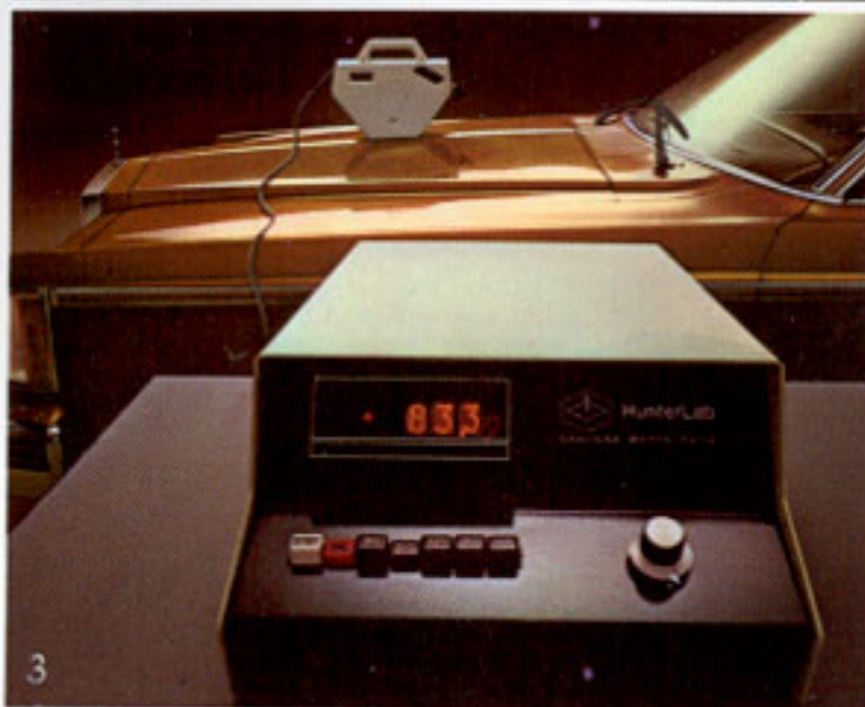
1. Every transmission is tested electronically. 2. Fifty electrical functions receive computerized inspection. 3. A special gloss meter evaluates the Clearcoat finish. 4. Every Versailles is test-driven on a road simulator.
