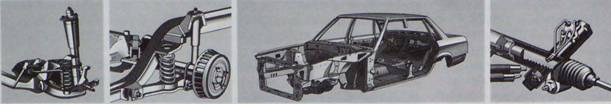
Wide-mount strut front suspension, 4-bar link coil spring rear suspension, Unitized body construction, variable ratio rack-and-pinion steering opt.
