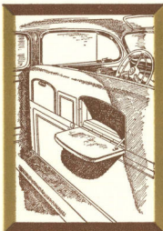
The back of the front seat of the 5-passenger Sedan contains two small compartments and lower compartment, long enough for a golf bag.
