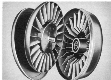
Disassembled view of the Chrysler Fluid Drive, showing the cover, runner and driver in their relative positions.
