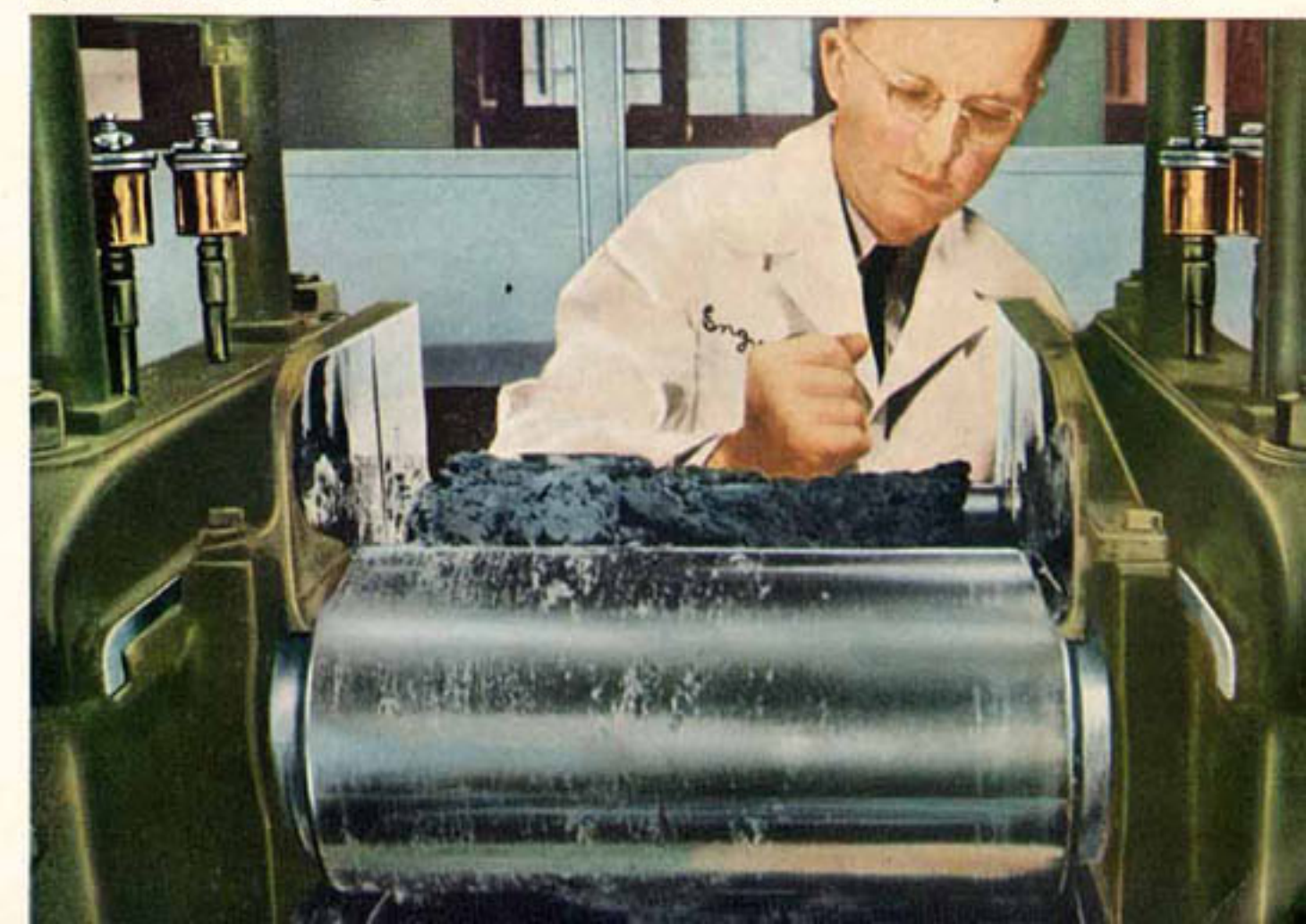
Ferrous Metals Laboratory (below, at left) is the scene of constant research and experimentation. Experimental Rubber "Mixing Bowl" (below)—Part of the ceaseless research in synthetic rubbers.
