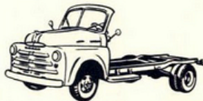
CHASSIS WITH WINDSHIELD COWL Available in 116" and 126" Wheelbases Single or Dual Rear wheels
