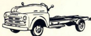
CHASSIS WITH FLAT-FACE COWL Available in 116" and 126" Wheelbases Single or Dual Rear wheels
