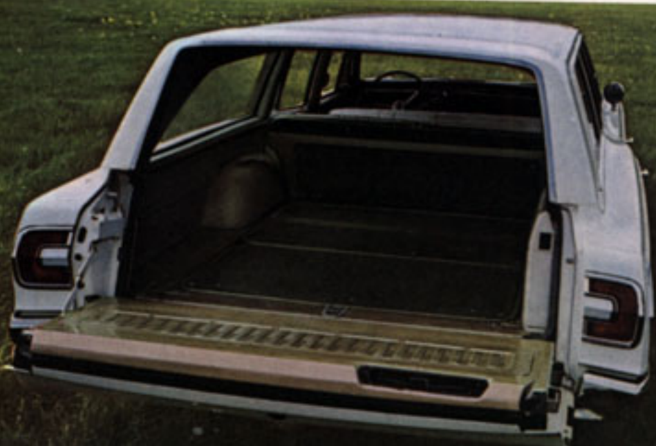
Standard equipment is a two-way tail gate, shown here on a Satellite Sport Wagon.
