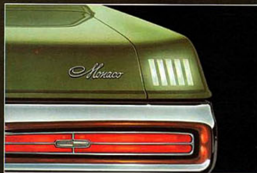
The vertical slots in the ends of the quarter panels shown above are the backup lights.
