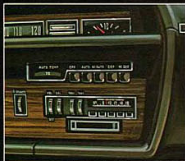
Monaco electric clock, AM radio with eight-track stereo-tape player, and air conditioning with automatic temperature control.
