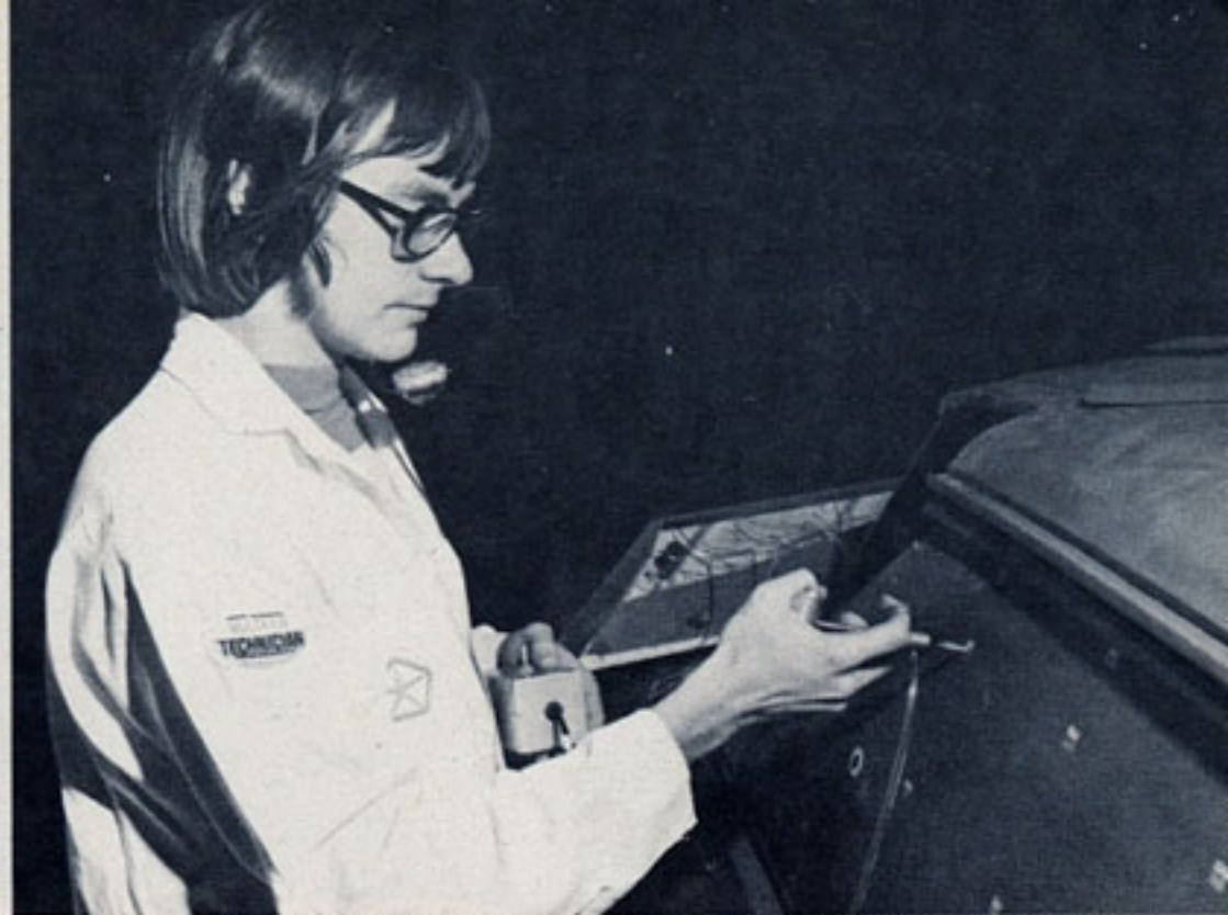
Checking instruments in a clay model to measure wind flow.
