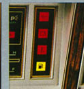
Warning light module—lights for low oil pressure, low voltage, high engine temperature, and low fuel.
