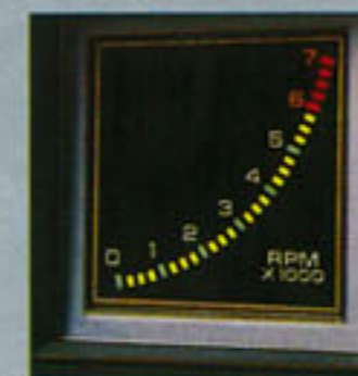
Analog tachometer with easy-to-read electronic display.
