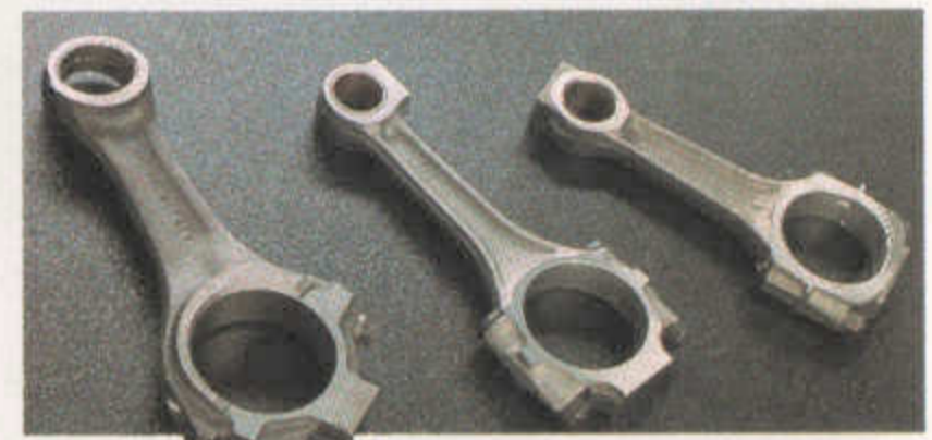
Connecting rods: Dodge Cummins Intercooled Turbo Diesel, Ford Navistar Diesel, Chevy/GMC Detroit Diesel.
