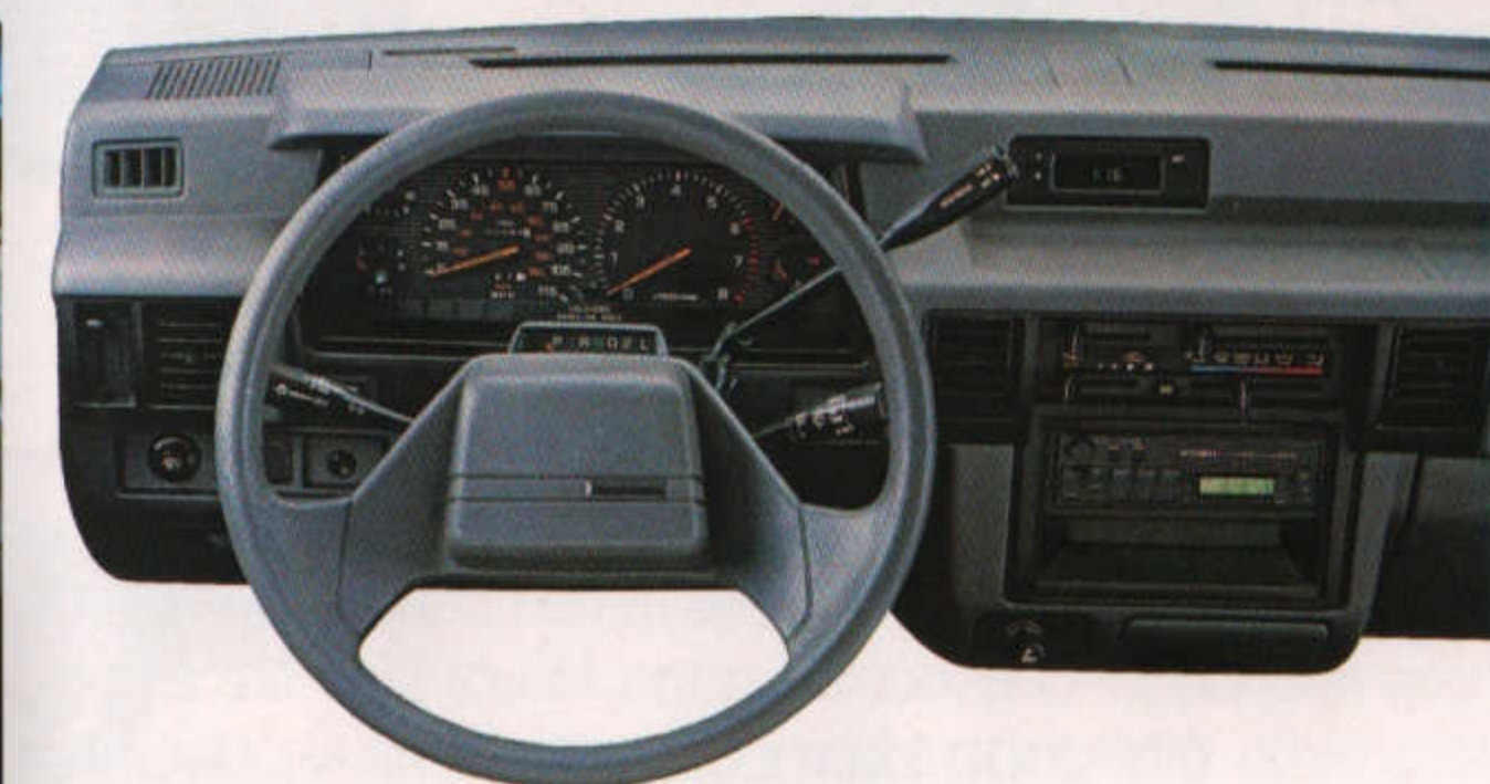
Ram 50 SE features a Sport soft-feel steering wheel and full instrumentation with a trip odometer and tachometer, plus gauges for fuel, voltage, temperature and oil pressure.
