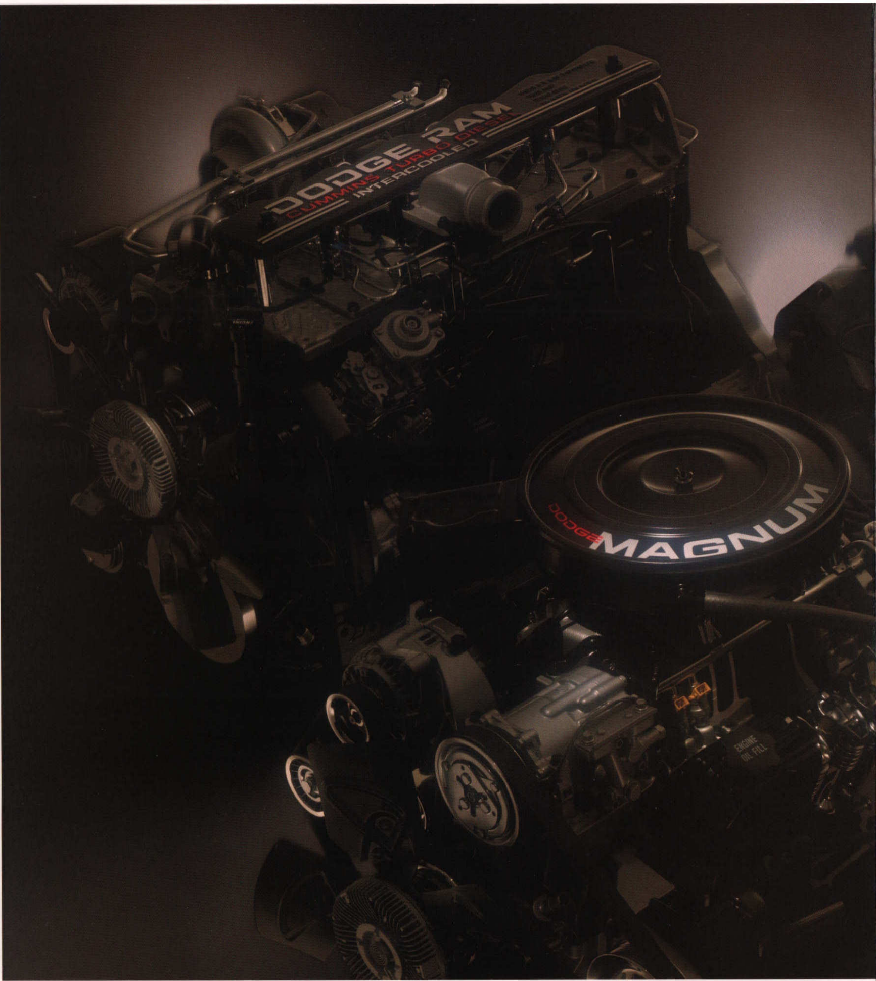
(top left) 5.9-liter I-6 Cummins Intercooled Turbo Diesel • 160 horsepower at 2,500 rpm. • 400 pound-feet of torque at 1,700 rpm.
