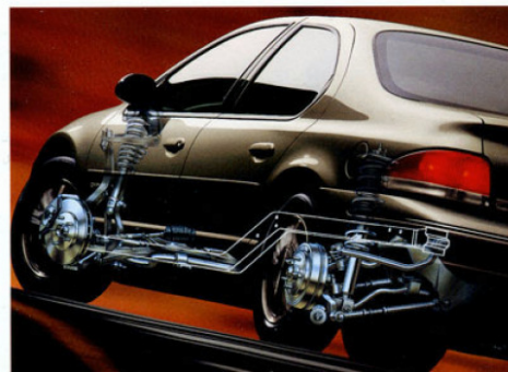
Cirrus' four-wheel fully independent modified double-wishbone suspension handles with precision.
